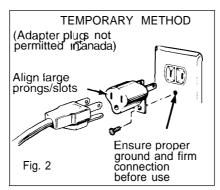
'he larger slot in the adapter must be aligned with the larger slot in the wall receptacle to provide proper polarity in the connection of the power cord.
